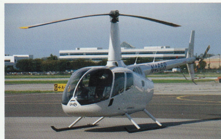
* The turbine R66 is still traditional Robinson: two-blade with a teetering rotor head.
