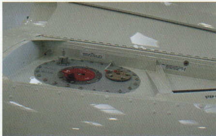
* R66 is the first machine from Robinson to use Jet A fuel. It addresses Avgas sourcing issues.
